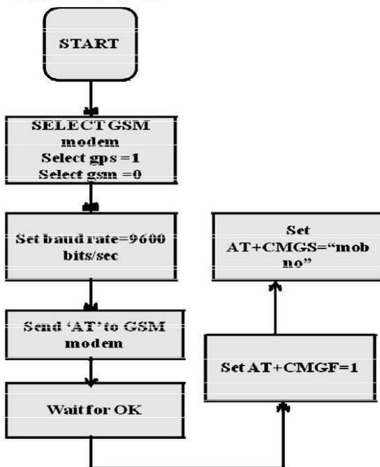
Fig 5: Flow chart of GSM
