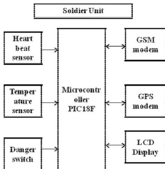
Fig.1: Block Diagram of Soldier unit
