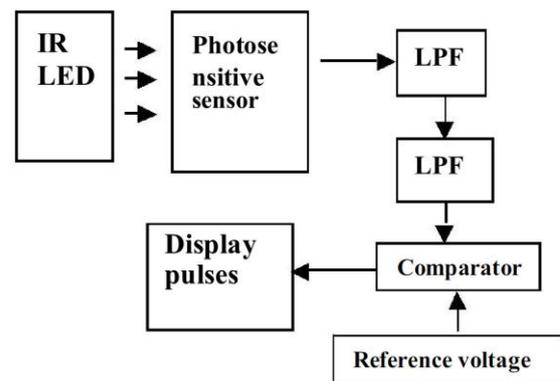
Fig.2: Block diagram of heart beat sensor.
